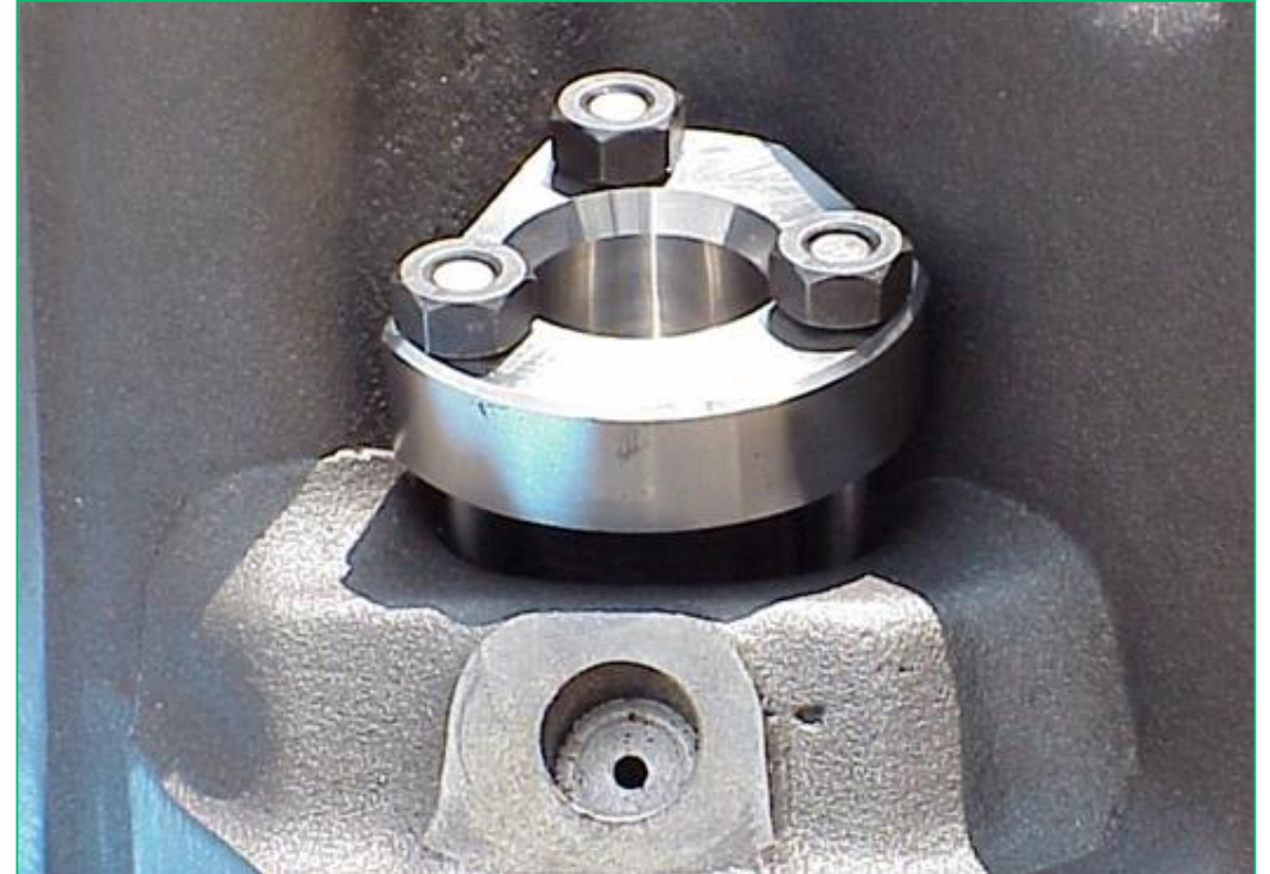
Pre-combustion chamber used on SGTD engines
